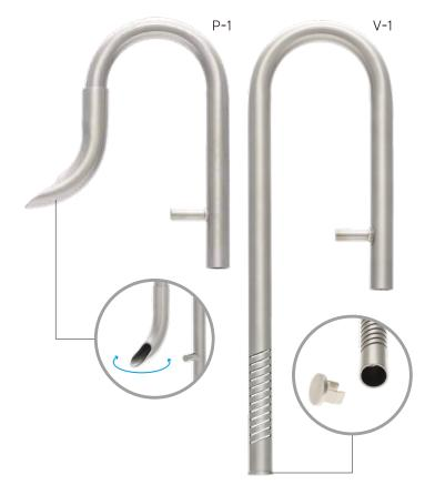
The stainless steel Metal Jet Pipe has been renewed to a new form with new functions. The new Metal Pipe Flow Series has an outflow nozzle that is horizontally movable, enabling the outflow direction to swivel to the left and right. This function enables us to create a water flow that is suitable for various layout styles. The inflow pipe has a detachable plug at the tip for easier maintenance.
